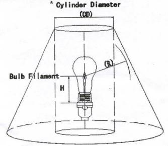
AT NO TIME SHOULD THE \* CYLINDER DIAMETER (CD) AND \*\*CRITICAL RADIUS (R) MEASUREMENTS OF YOUR ALTERNATE SHADE BE LESS THAN THE MEASUREMENTS NOTED BELOW, AS THIS MAY CAUSE A FIRE HAZARD
