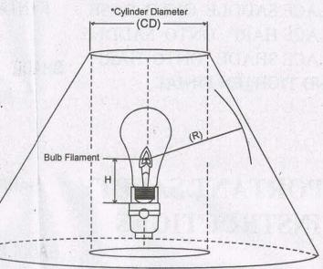
AT NO TIME SHOULD THE \*CYLINDER DIAMETER (CD) AND \*\*CRITICAL RADIUS (R) MEASUREMENTS OF YOUR ALTERNATE SHADE BE LESS THAN THE MEASUREMENTS NOTED BELOW, AS THIS MAY CAUSE A FIRE HAZARD.
